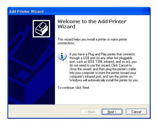
Click Next and select Local Printer, make sure the Automatically detect and install my Plug and Play printer check box is NOT checked. Then click Next.
